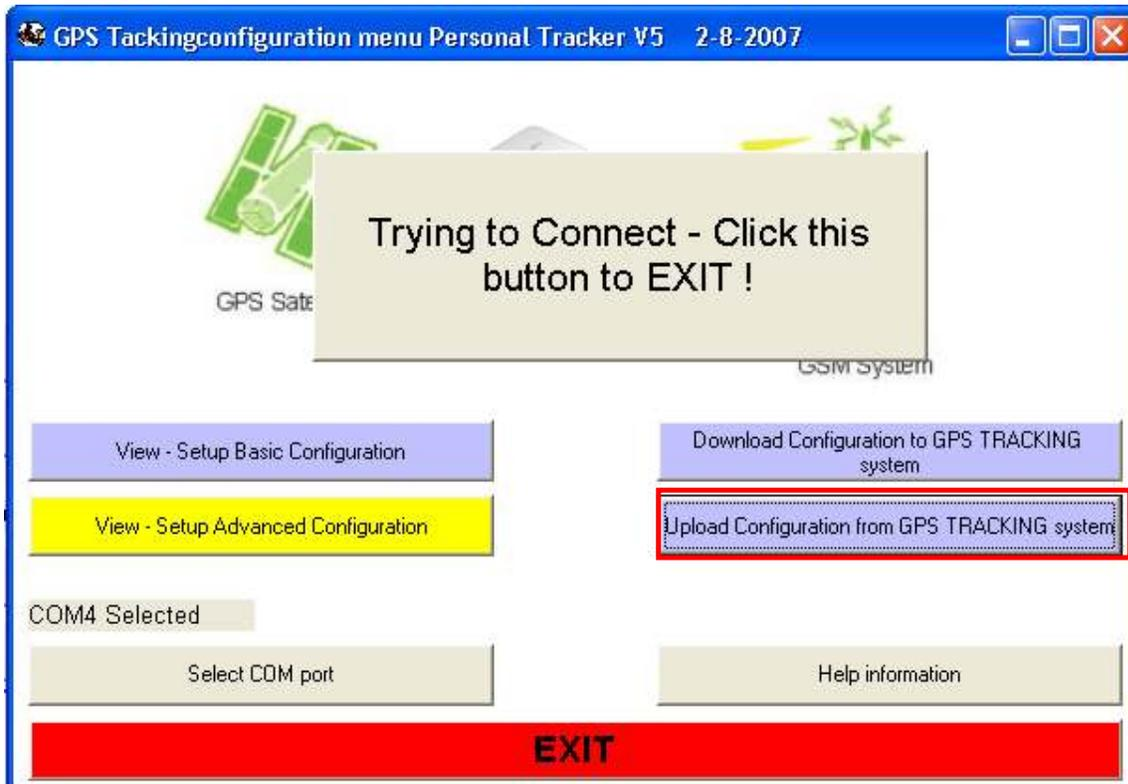
Always upload the current configuration from the WTGAT first. This way it is easy to configure and the setup the unit. You must use the correct WTGAT firmware version. The configuration file cannot be uploaded if the version is incorrect.
